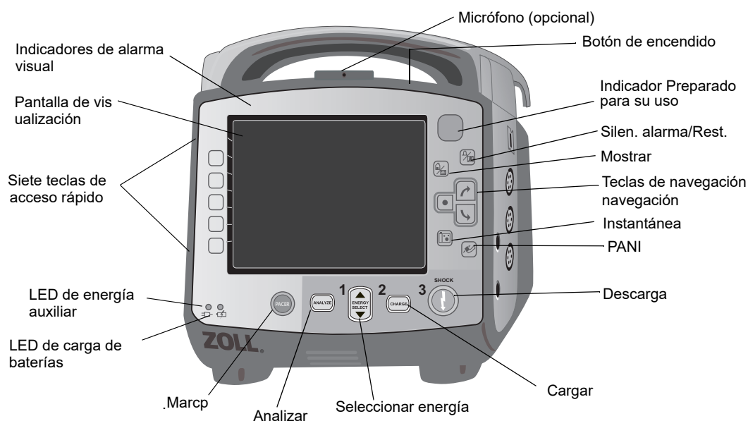
Figura 2-1. Panel frontal de X Series Advanced
