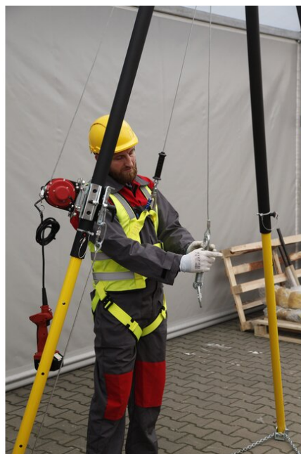
RUP506 winch installed on a TM15 tripod leg
